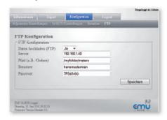
The CSV files are automatically uploaded to an FTP server. The EMU M-Bus Logger website then allows you to select and configure your FTP server.
